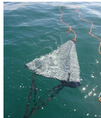
Figure 9: Photo d'une ancre flottante (Source: [http :
